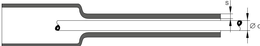
d: Nominal diameter (according to the object to be covered)
